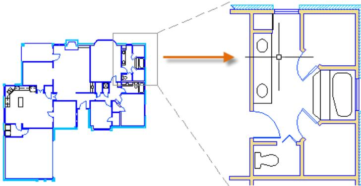
**Note:** If you cannot zoom or pan any more, type REGEN in the Command window and press Enter. This command regenerates the drawing display and resets the extents available for panning and zooming.
