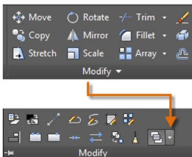
The draw order options that are listed include sending all hatches to the back, all text to the front, and so on.
